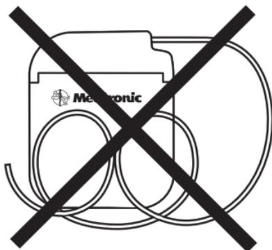
**Figure 3.** Wrap excess extensions or leads around the perimeter (or behind) the neurostimulator.
